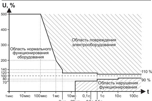
Рис. 1. Кривая работы электрооборудования ITIC (CBEMA), ([http://www.home.agilent.com/upload/cmcc\\_upload/All/1.pdf?&cc=UA&lc=eng](http://www.home.agilent.com/upload/cmcc_upload/All/1.pdf?&cc=UA&lc=eng)).
