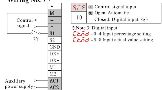
※Note 1: When the contact is disconnected output will be according to CT.MD control mode.
